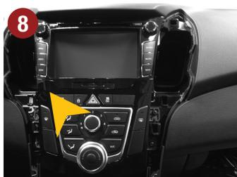
8.) Before you complete the installation, make a function check. Please note that it may take up to 15 minutes, until a GPS signal can be received outside.
