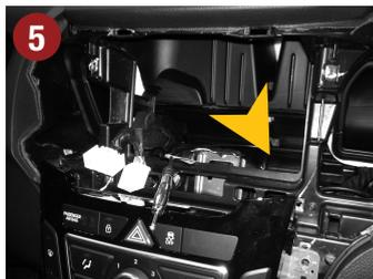
5.) Lay the connection cable sets of new ESX device (refer to page 4-5) inside the vehicle to the desired location.
