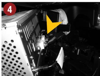
4.) Then pull out the radio unit from the bay and disconnect all cable plugs from the device.
