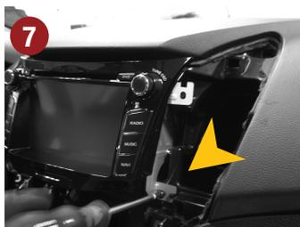
7.) Then slide the new ESX device carefully into the radio bay. Ensure that the new device sits proper in the previously installed mounting frame.
