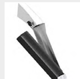
Battery fully integrated into the frame
