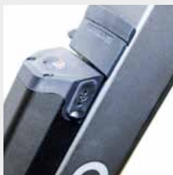
Hydroformed frame with integrated battery
