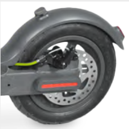
Mechanical rear disc brake
